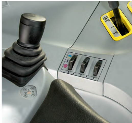
Up to seven remote valves can be operated.
