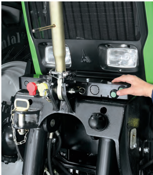
The integrated front hydraulic system and front PTO, available options.
