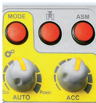
The controls for changing the driving strategy are in the armrest.
