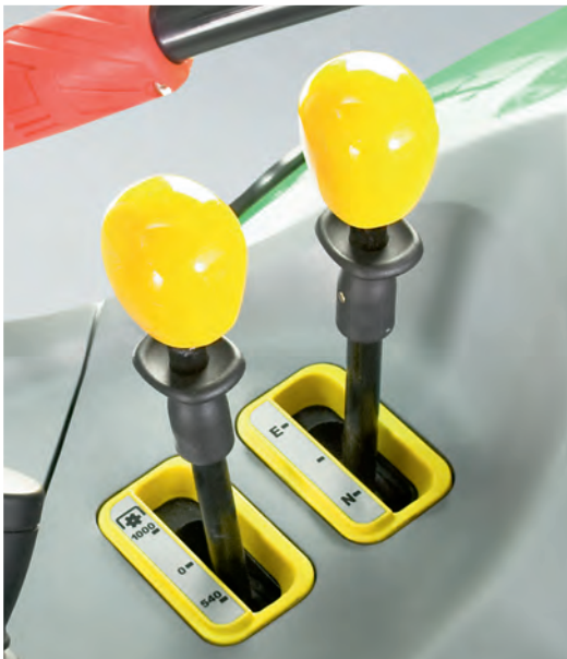
The PTO speeds can be conveniently pre-selected.
